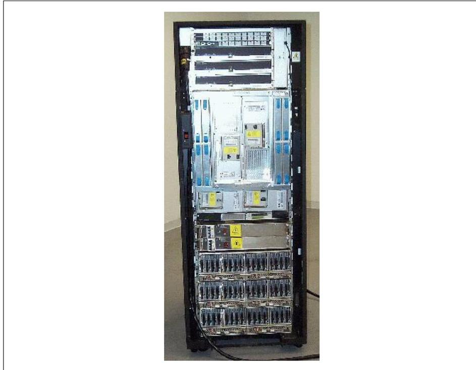
*Figure 2-8 The p670 with three I/O expansion drawers*
