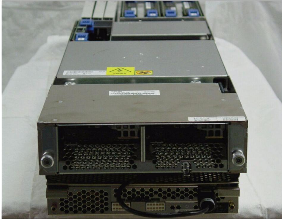
Figure 2-4 The p655 front view without covers and SCSI disks
